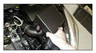
5. Pull the air filter housing straight up and remove it from the vehicle.
