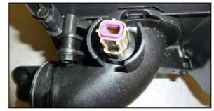
6. Lift the small locking tab and rotate the Inlet temperature sensor counter clockwise and remove the sensor. Remove the O-ring from the sensor.
