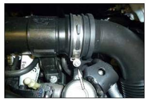
4. Loosen the clamp that secures the upper intake tube to the turbo inlet pipe and then remove the upper intake tube.
