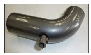
7. Install the inlet temperature sensor onto the AEM® intake tube using the provided grommet.
