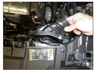
12. Remove the fresh air intake duct from the core support.
