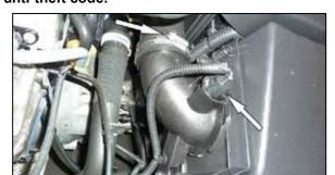
2. Disconnect the inlet air temperature sensor electrical connection. Then loosen the hose clamp that secures intake filter tube to the intake tube.
