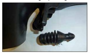
8. Remove the factory air filter housing mount from the factory air filter housing.
