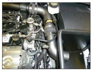
15. Install the two AEM® intake tubes and hump hose coupler into the coupler at the turbo inlet and through the heat shield as shown, do not
