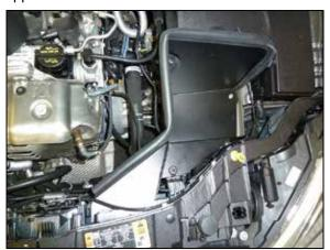
13. Install the heat shield into the factory air filter housing mounts.
