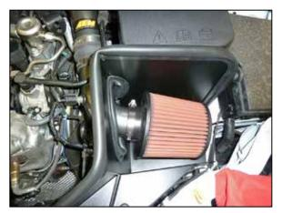
16. Install the AEM® air filter onto the intake tube and secure with the provided hose clamp. Reconnect the inlet air temperature sensor electrical connection and then adjust the tube and filter for best fit then secure with the provided hose clamps.
