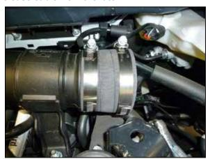
14. Install the provided hose coupler onto the turbo inlet pipe.
